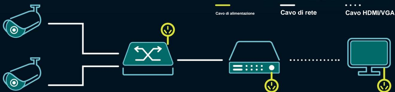
**Telecamera IP + switch PoE + NVR automatico + Monitor**
